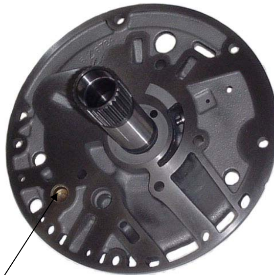
Location of cooler bypass plug
